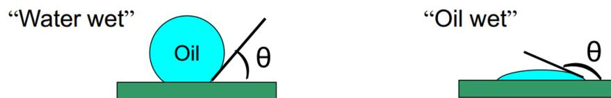
Figure 3.2: Wettability and Contact Angle
